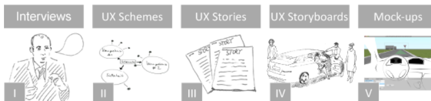
Fig. 1. The five steps of the design workflow.
