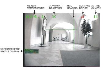
Fig. 5. RoBrno's interface, a strongly simplified interface, contradictory to the INEEL interface, presented in [4].
