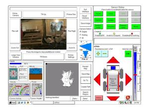
Fig. 2. The INEEL interface for their robotic system [5].
