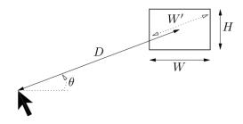
Fig. 1: Fitts' Law task in two dimensions. [4]
