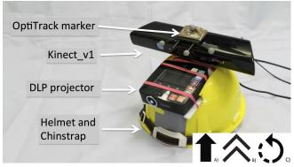
Figure 2. The HelmetPickAR order picking helmet and the arrows that can be displayed to navigate the participant.
