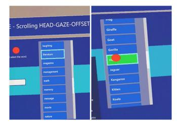
Figure 3: The *Head-Gaze Offset* interaction method. The left side shows the scrolling with the head direction above the middle of the list and the gaze below the head direction. The right side shows the selection of a list item by placing the red dot and the gaze onto the list item. The red dot shows the head direction with a  $9^{\circ}$  offset to the left.
