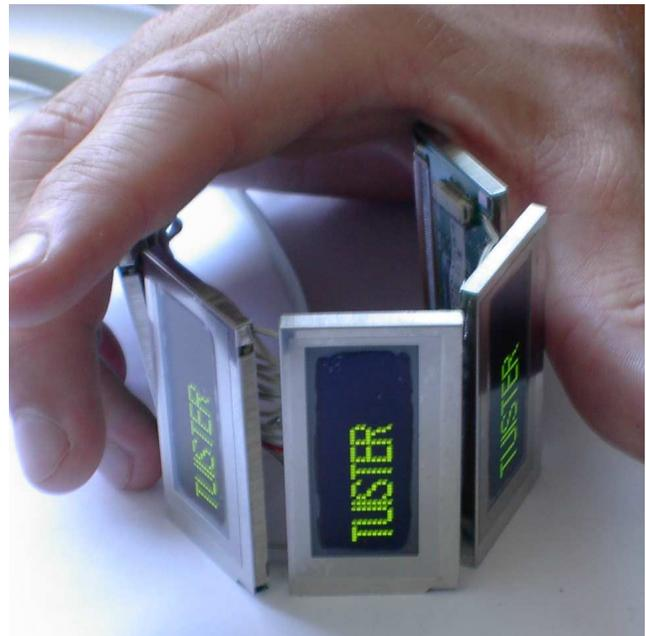
Figure 4: The display part consists of six organic displays in a hexagonal arrangement
