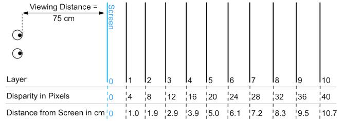
**Figure 2:** Layer positions applied in the user study. The distances between the screen layer and each depth layer are given in pixels and cm.
