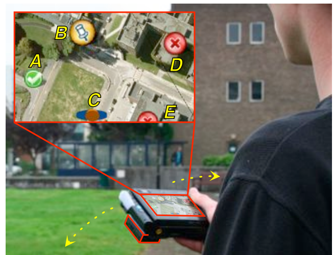
Figure 4: The visual browsing comparison system, showing the on-screen display (inset). Point A has previously been selected, point B is currently being pointed at by the user and is activated. Point C represents the user at their current position. The two remaining points, D and E, have not yet been visited.
