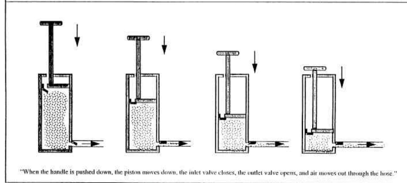
"When the handle is pushed down, the piston moves down, the inlet valve closes, the outlet valve opens, and air moves out through the hose."
