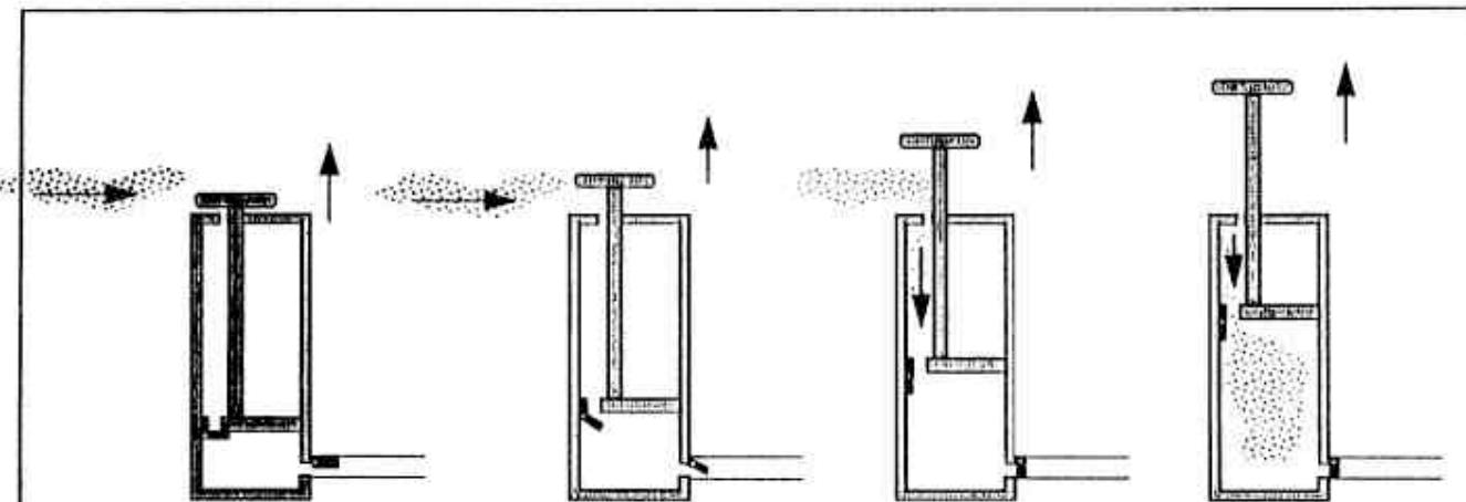
"When the handle is pulled up, the piston moves up, the inlet valve opens, the outlet valve closes, and air enters the lower part of the cylinder."
