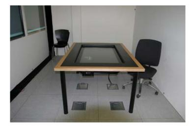
This is a picture of the Tabletop your prototype will be running on. The **resolution** is  $1360 \times 768$  pixel. The **display area** is  $102 \times 57$  cm. The dimension of the whole table is  $155 \times 110$  cm. Here are the dimensions from a top-down perspective in detail:
