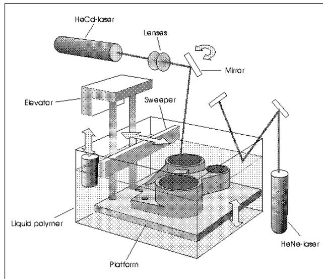
FIGURE 1. A schematic drawing of an SLA.
