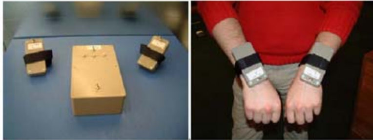
Fig. 1. (a) GentleGuide control unit and wrist devices (b) GentleGuide worn by a participant
